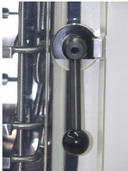
Fig. 17: Example of a door locking system of the loading door; here: door stop (left side)
