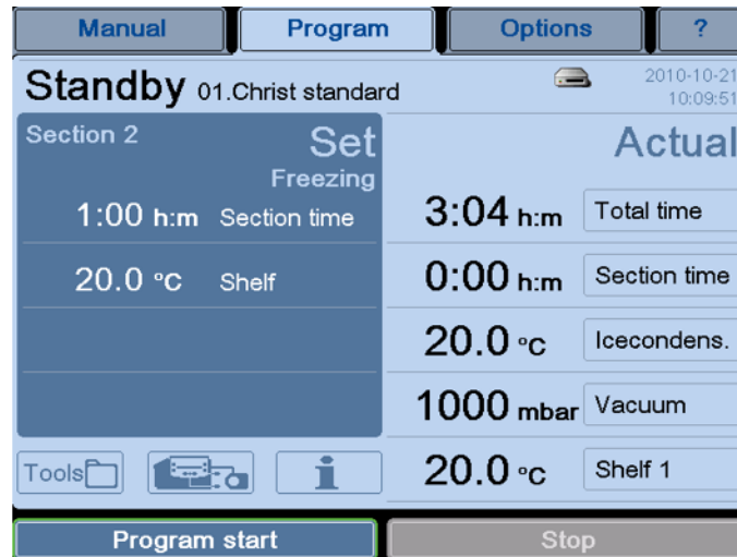
Fig. 74: The freeze-drying process can be started with the aid of the button "Program start".
