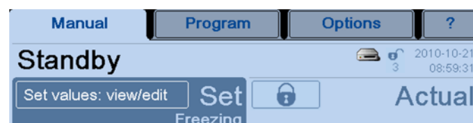
Fig. 47: Countdown of the password timer and the button with the lock symbol
